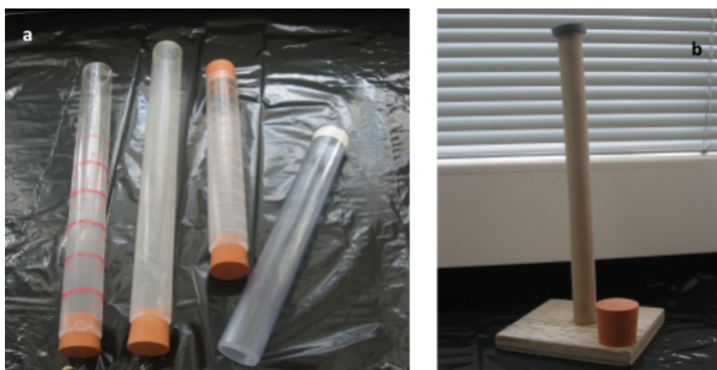
Figure 3. a) Corers with rubber stoppers and b) core plunger for shallow subtidal sampling.
